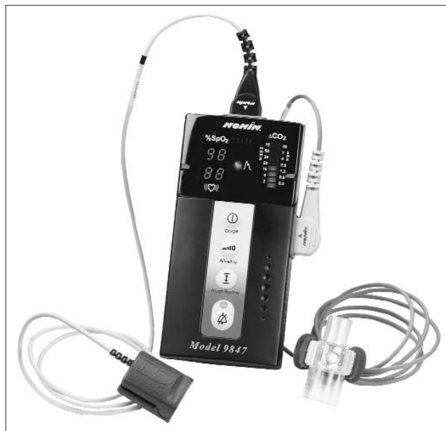
FIGURE 6 Capnometers provide a numeric measurement of the concentration of CO 2 present in the exhaled air. These devices are available as portable units or as add-ons to bedside monitors.
