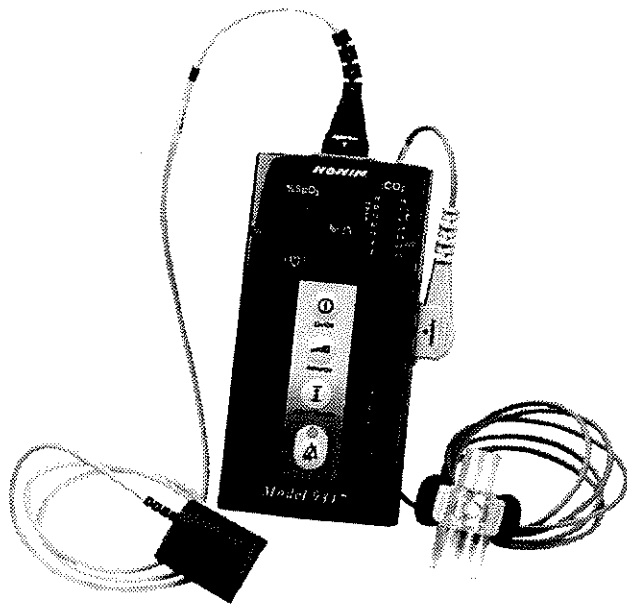
FIGURE 9 ■ Capnometer for measuring EtCO 2 ; also measures heart rate and SaO 2 .
